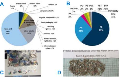
Fig. 1: Analysis of marine litter and production of marine litter-derived MPs. A: composition of litter items, B: polymer composition of litter, C: marine litter subcategories before milling, D: PTX001, marine litter-derived MPs - a representative mixture of polymers in the environment. Picture credits: WMR, SINTEF and Carat GmbH.
