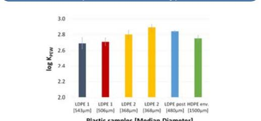
Fig. 5: PE-water partition coefficients of naphthalene on PE from different origins. The origin of "LDPE 1" and "LDPE 2" are pristine pellets by two different producers; "LDPE post" is recycled post industrial waste; "HDPE env." is beached yellow fish box.
