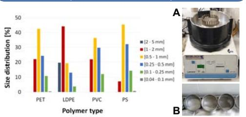
Fig. 3: Size distribution of plastic particles (PET, LDPE, PVC and PS) after grinding using Ultra centrifugal mill + N<sub>2</sub>(liq). A: Ultra centrifugal mill B: Plastic particles after grinding. Picture credits: AMU-MIO.
