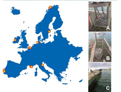
Fig. 2: Long-term field tests in PLASTOX WP1. Red circles indicate the location of the marine stations for a long-term field test. A: Plastic samples in a metal cage; B: The metal cage to be exposed to the marine environment; C: A deployment site in Belgium. Picture credits: UGent
