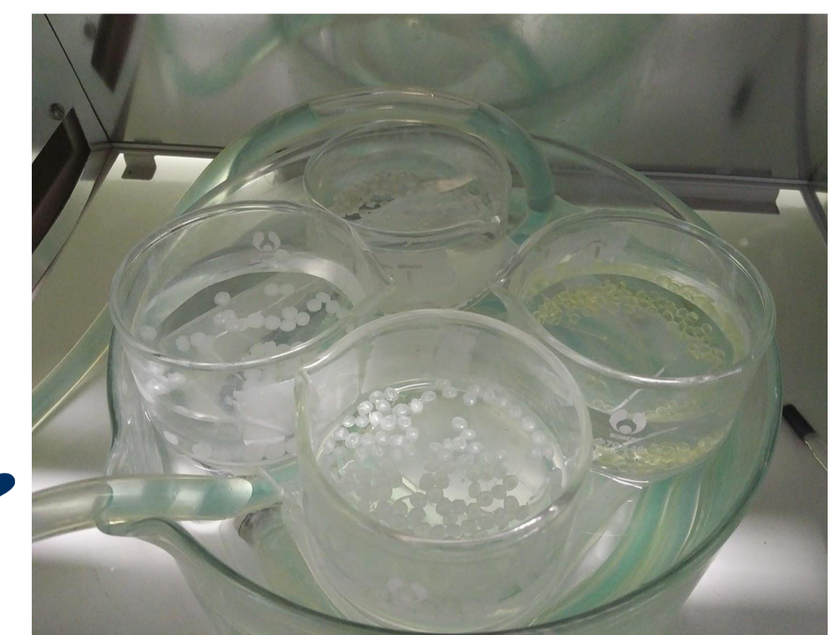
Figure 2. Artificial aging of PE, PP, PS and PET granules
